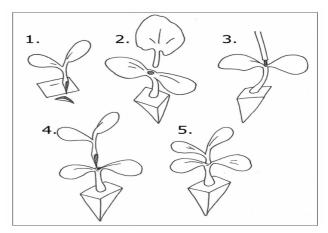
**Splice grafting:** This method is widely used by growers and can be performed manually or with machines for most cucurbit and solanaceous vegetable crops.
